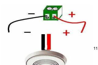
3. Sink mode (Resistance signal)—IN5 & IN8: can be connected to magnetic reed switch as the follow figures
