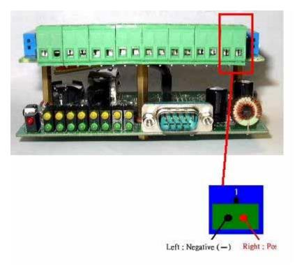
**NOTE**: Because of the polarity protective function, it won't damage the product if user reverse the polarity in installation. But it will cause the product cannot work properly
