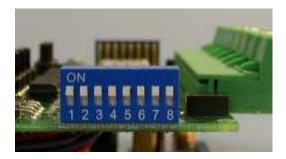
Then user can setup the Dry/Wet contact in LEFT switch :
