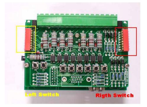
There are two switches in 9211. Please arrange all the setup to ON in the Right Switch.
