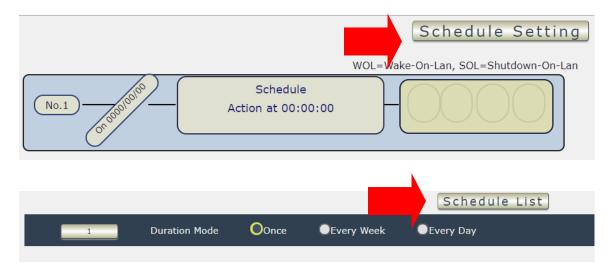
The schedule allows you to control the power outlet turn ON, OFF, Cycle, WOL, SOL or Reboot at the assigned time user arrange in schedule
