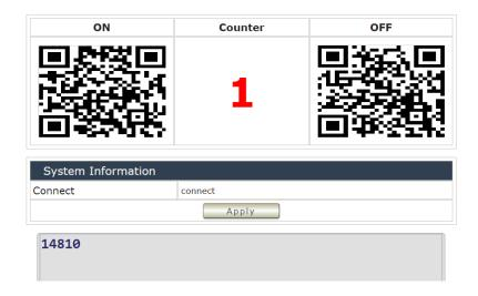
Scanning on and off QR code will trigger the IO control, and will show their command code below.
