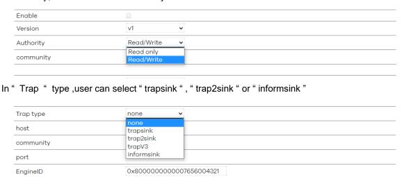
SNMP Version: IP9855 PRO provide V1, V2 and V3 version. V1 and V2 remain the same settings, when you switch to V3, user can see the difference in the second picture.
